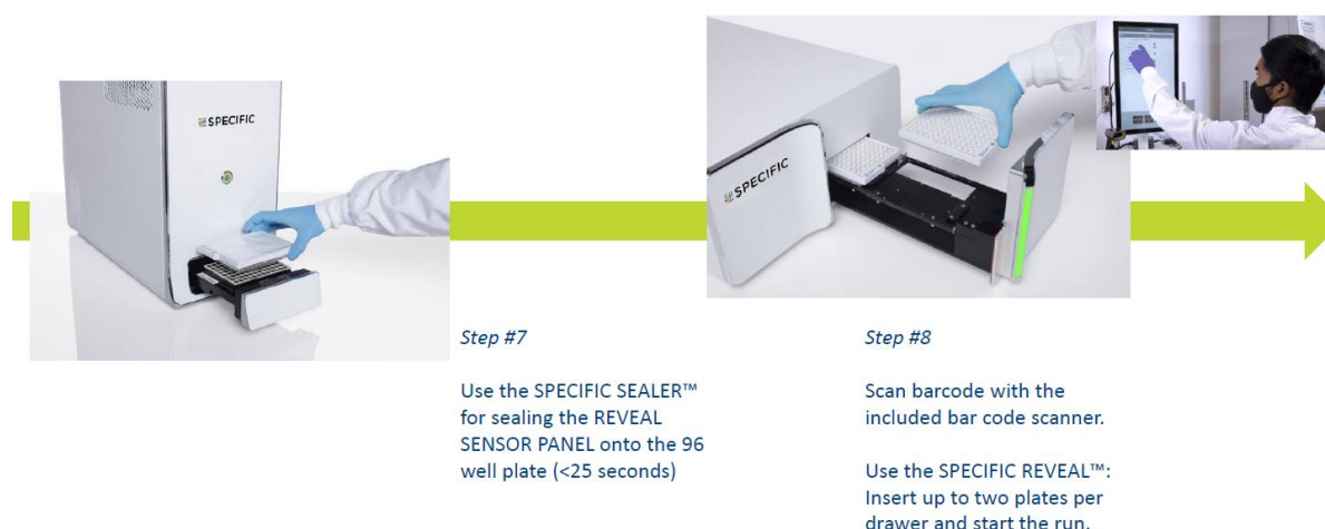
Figure 6 Second part of the sample preparation for the VITEK® REVEAL™ AST GN01 panel. The first part of the procedure is depicted in Fig. 5.
